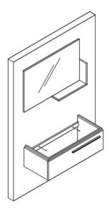
5. Fill up silicon between the bench and wall
