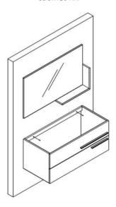
5. Fill up silicon between the bench and wall.
