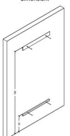
3. Place the cabinet to wall as balanced. Install the iron hanger to the wall and cabinet to make the cabinet fix.
