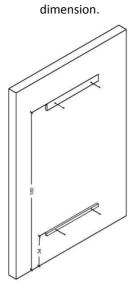
3. Place the cabinet to wall as balanced. Install the iron hanger to the wall and cabinet to make the cabinet fix.
